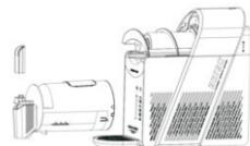
2).Assemble the drip tray, residual liquid box, and stirrer.
